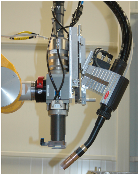
Figure 6.14: Photo of the HLG head, consisting of a BEO D70 Trumpf laser welding head, combined with a Fronius Robacta Drive CMT torch.
