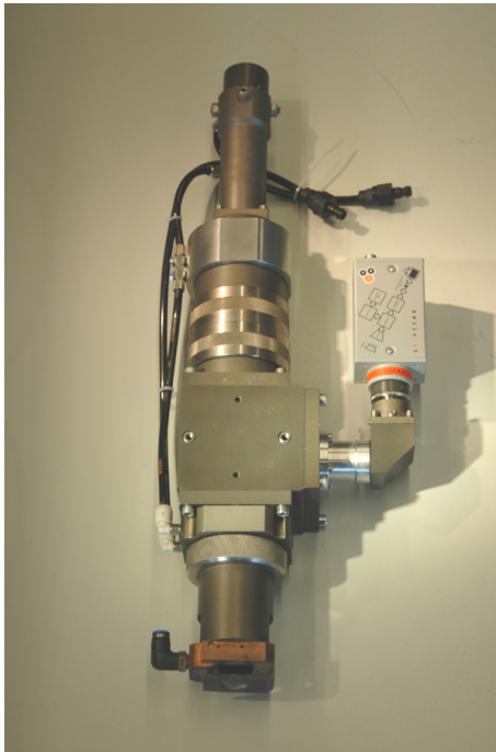
Figure 3.9: Photo of the BEO D70 Trumpf laser welding head, together with the PixeLINK PL-A741 CMOS camera.
