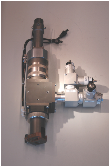
Figure 2.10: Photo of the LWM sensors attached to the BEO D70 Trumpf laser welding head.
