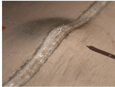
Figure 6.32: Photograph of a AA5182-O/H111 weld sample after the Erichsen Cupping test. The black line on the right side is a shadow of the Erichsen Cupping test apparatus.
